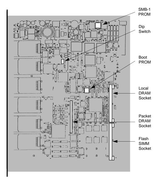
Figure 2-5. User-Accessible Components
